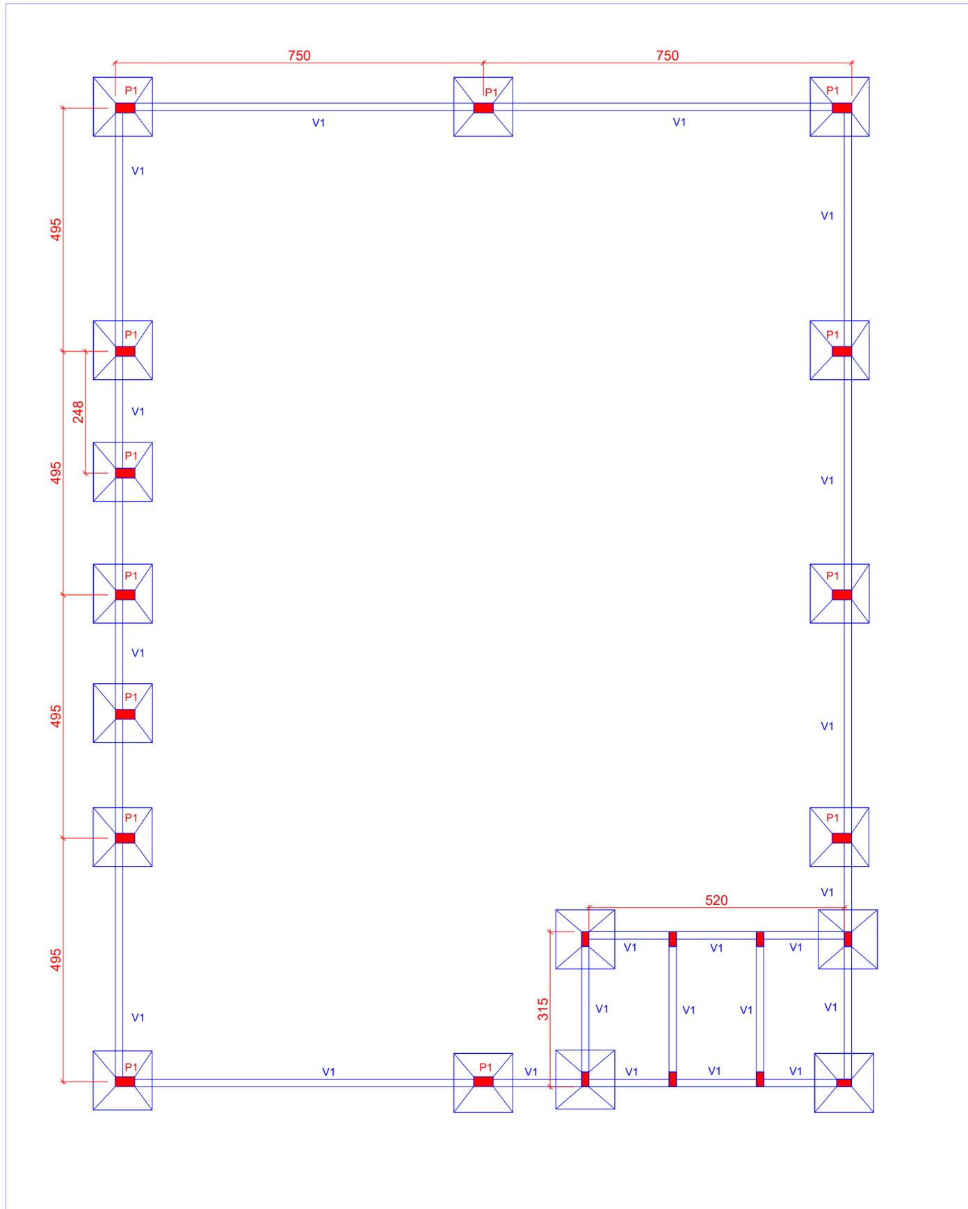
ESTRUTURAS (SAPATA, BALDRAME, PILARES, VIGA CINTA)
